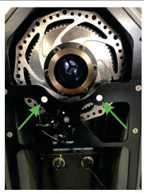
**Step C35: Reassembly**In the CALIPER SUPPORT FRAME there are two clearance holes as shown in this photo.
